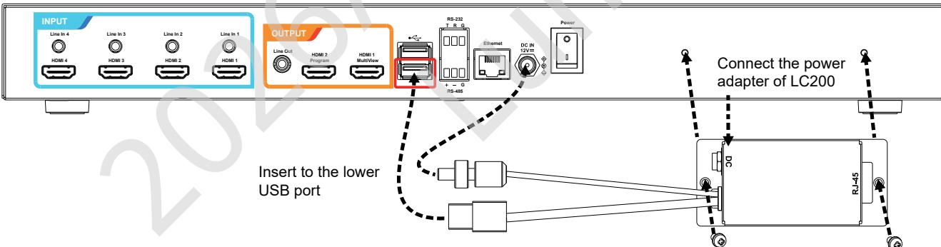
2. Use the CAT6 network cable for connection (the length shall not exceed 30 meters)
