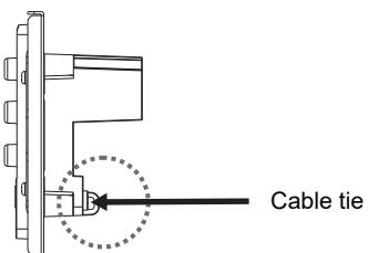
4. Install the control box on the wall
