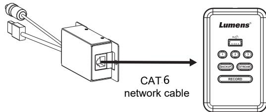
3. Pass a cable tie through the mounting hole to secure the network cable onto the LC-RC01 control box
